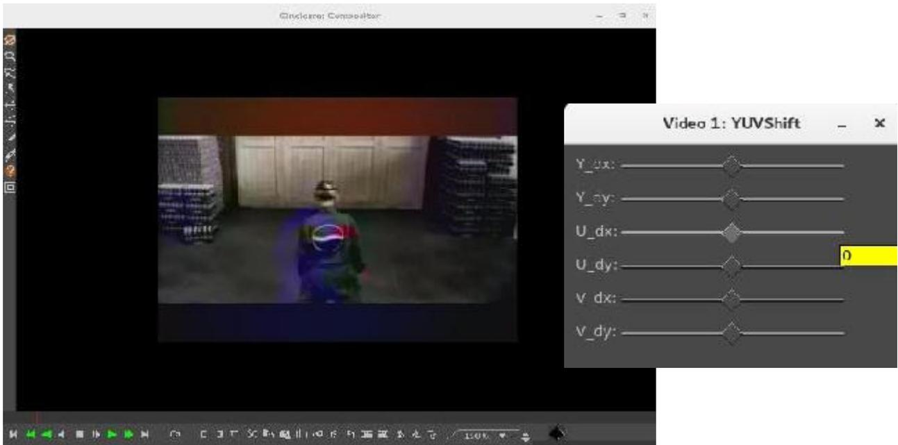
A corrected video image is shown in the screenshot below. Now the red and blue colors are correctly aligned. Note how U\_dx is now at +20 and V\_dx is now negative to realign the image.
